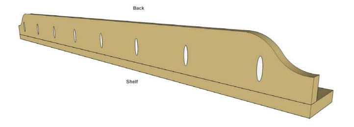
**Step 4:** Cut one piece of Front Molding to length, as shown in the cutting diagram. Note that each end gets mitered at 45° to allow the molding to wrap around the Shelf. Also cut two pieces of End Molding, mitering one end of each piece where it will join to the Front Molding.
