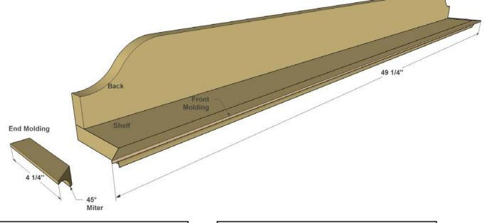
**Step 5:** Glue the Front Molding and End Molding in place on the Shelf. Take care to align the miters. To hold the pieces in place as the glue sets, use masking tape.
