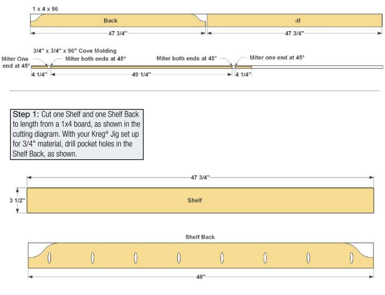
Step 2: Lay out the curved shapes on each end of the Shelf Back using a compass. You'll set it to a 2 3/8" radius for the outer curves, and to 2 3/4" for the inner curves. If the two arcs don't meet exactly when you lay them out, that's okay. Just connect the lines. Cut the shapes with a jigsaw, and then sand them smooth.
