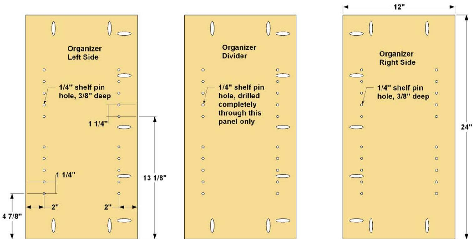
**Step 16:** Cut one Left Organizer Side, one Organizer Divider, and one Right Organizer Side to size from 3/4" MDF. Then you need to drill shelf pin holes in these parts. Before you do this, mark the bottom edge of each piece so you get all of the holes positioned correctly. Note that the Divider needs holes in both faces. After you drill the shelf pin holes, drill pocket holes, as shown, with your pocket hole jig set up for 3/4" material.
