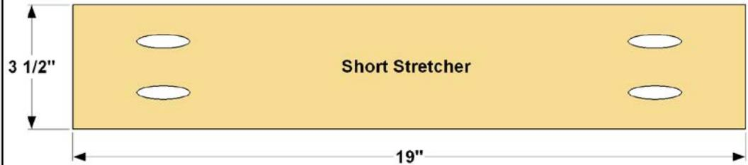
**Step 2:** Assemble the bench ends by attaching the Short Stretchers to the Legs using 2 1/2" pocket hole screws, as shown.
