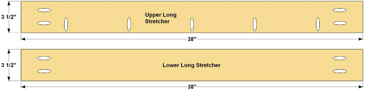
**Step 3:** Cut five Long Stretchers to length from 2x4 boards, as shown in the cutting diagram. With your pocket hole jig set up for 1 1/2" material, drill pocket holes in three of pieces to create three Upper Long Stretchers. Then, create two Lower Long Stretchers by drilling those pocket holes where shown.
