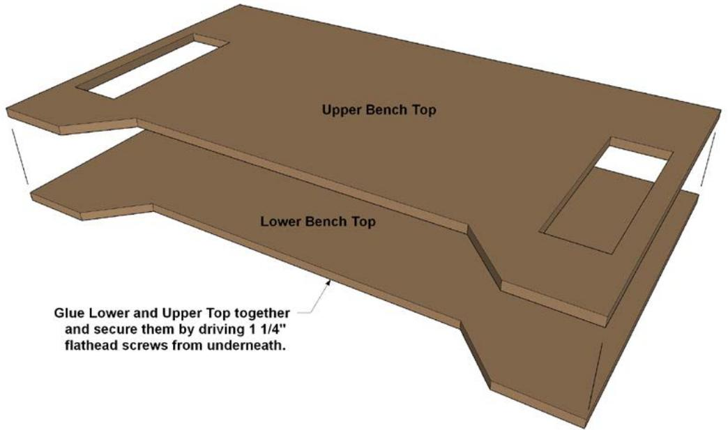
**Step 8:** Now you can attach the top assembly to the bench base using 1 1/2" pocket hole screws. Make sure the top assembly is flush with the bench Legs at the back, and that the top assembly overhangs equally on each end.
