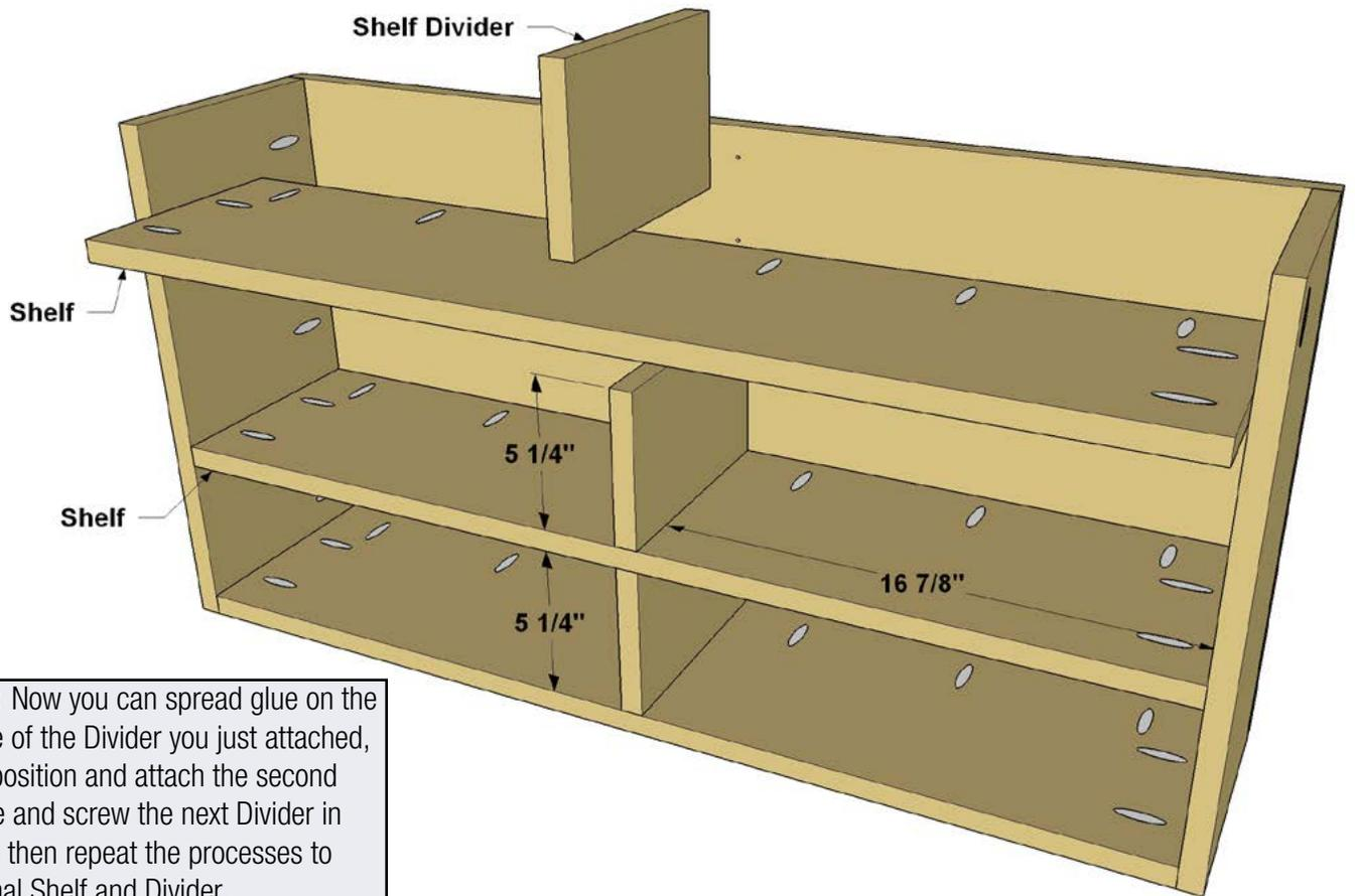
**Step 13:** Now you can spread glue on the other edge of the Divider you just attached, and then position and attach the second Shelf. Glue and screw the next Divider in place, and then repeat the processes to add the final Shelf and Divider.
