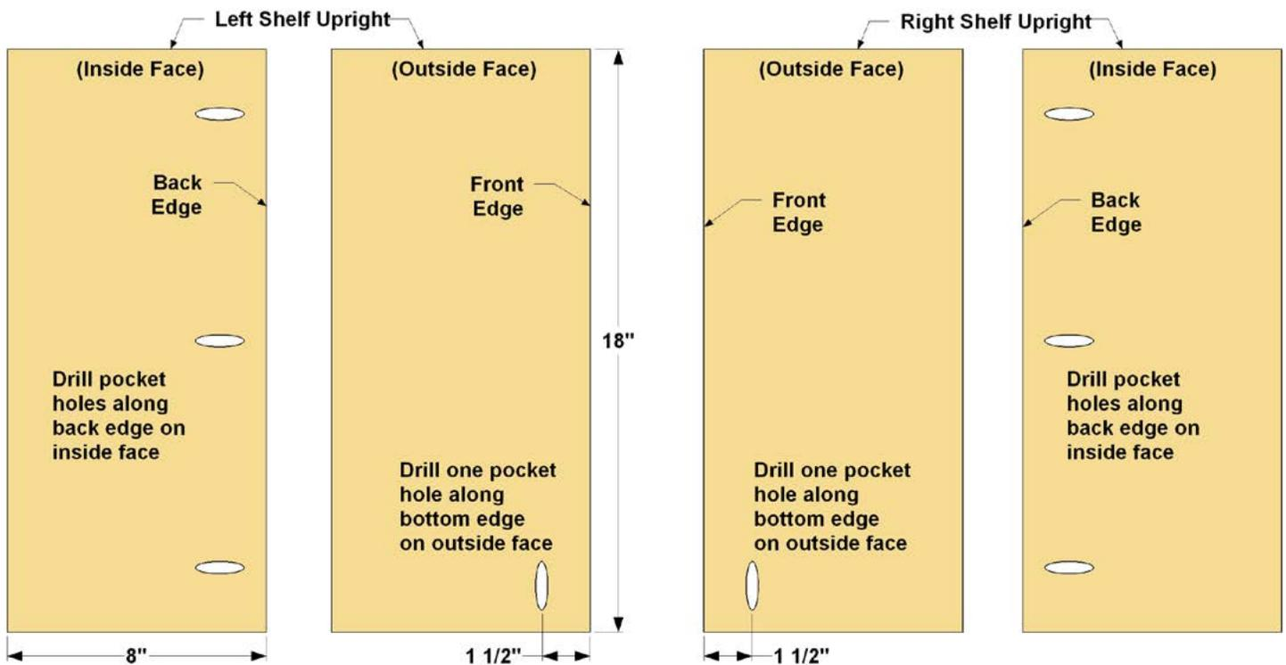
**Step 10:** Cut two Shelf Uprights to size from 3/4" MDF, as shown in the cutting diagram. Then drill pocket holes where shown with your pocket hole jig set up for 3/4" material. Note that you need to create a "matched pair" of uprights. You'll drill pocket holes along the back edge of each one on the inside face. Then you need to drill one pocket hole in the outside face of each upright, as shown.
