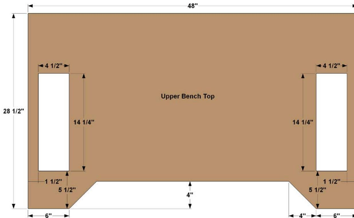
**Step 6:** Cut one Upper Bench Top to size from 3/4" MDF, as shown in the cutting diagram. Then lay out and cut the recess along the front edge using a jigsaw. Next, lay out and create the tray openings. Start by drilling a hole at each corner, then cutting along the lines with a jigsaw.
