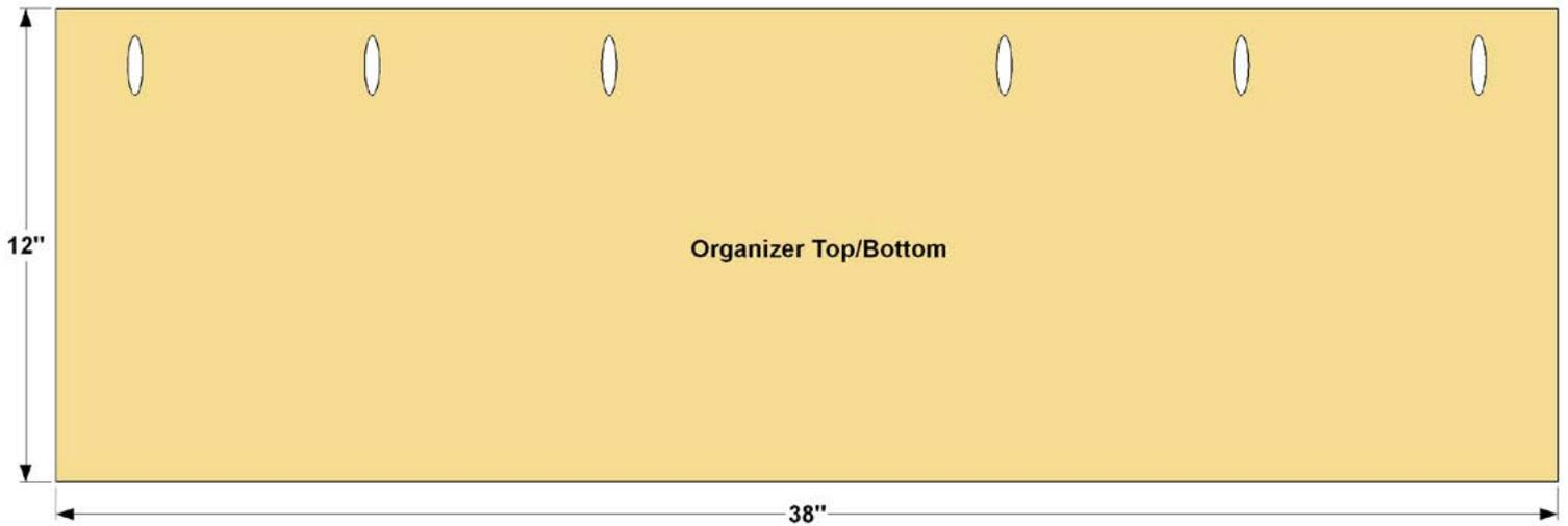
**Step 15:** Cut one Organizer Back, one Organizer Top, and one Organizer Bottom to size from 3/4" MDF, as shown in the cutting diagram. With your pocket hole jig set up for 3/4" material, drill pocket holes in the Organizer Top and Bottom as shown.
