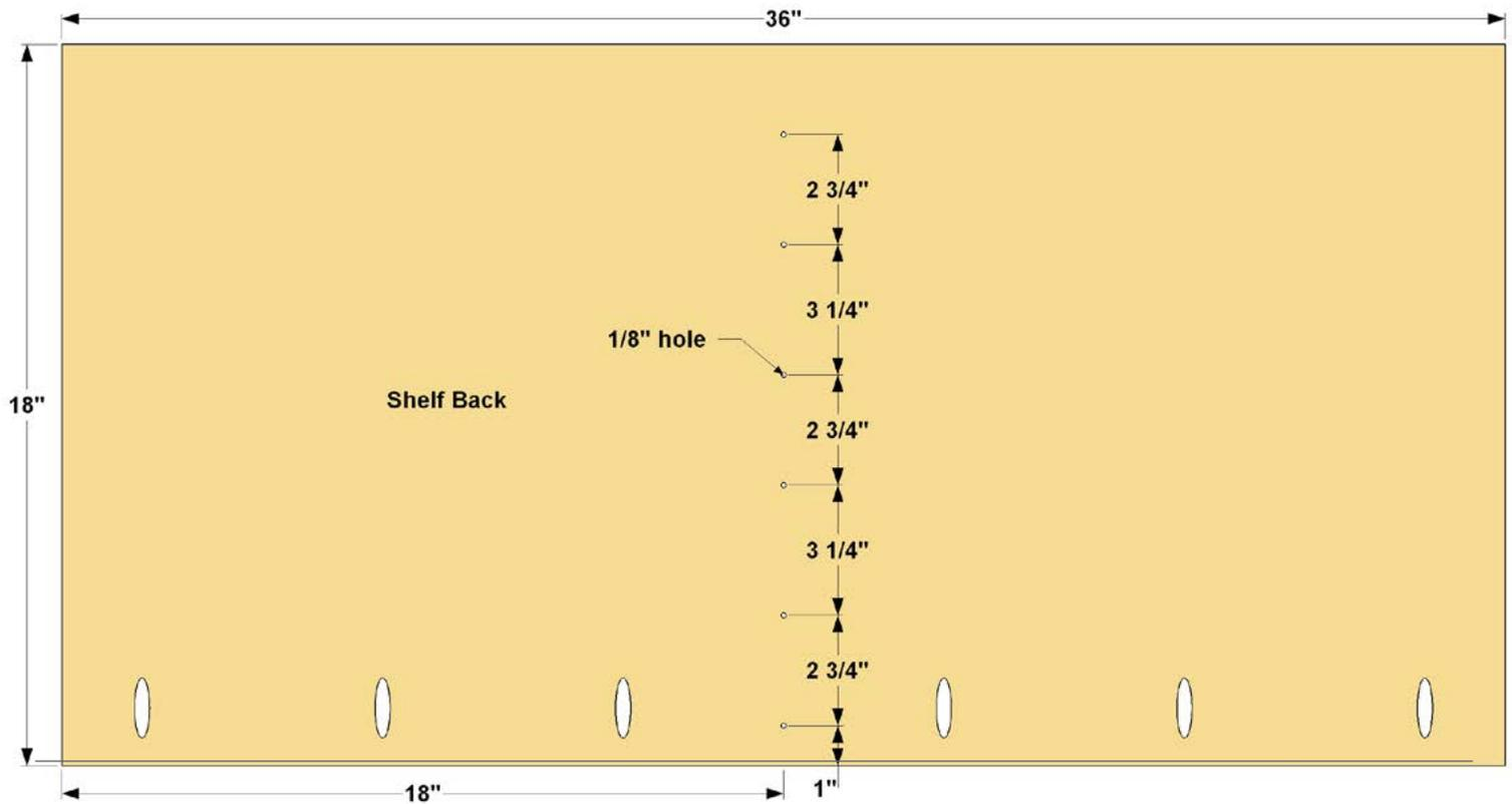
**Step 11:** Cut a Shelf Back to size from 3/4" MDF, as shown in the cutting diagram. Then drill pocket holes where shown. After that, you need to drill a row of holes through the Shelf Back, as shown. These will be used for screws that attach the Shelf Dividers.
