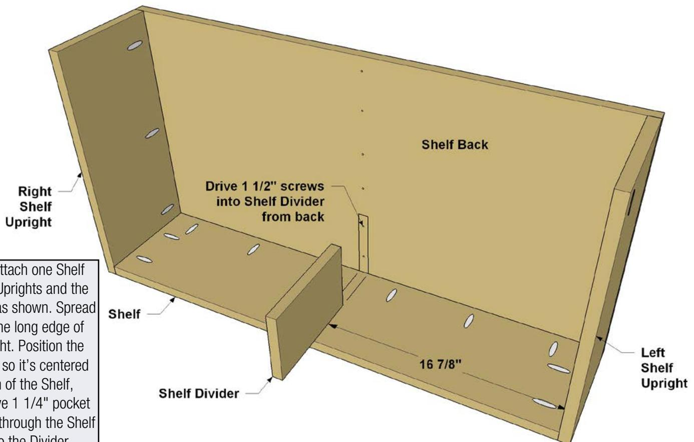
**Step 12:** Attach one Shelf to the Shelf Uprights and the Shelf Back, as shown. Spread glue along one long edge of a Shelf Upright. Position the Shelf Divider so it's centered on the length of the Shelf, and then drive 1 1/4" pocket hole screws through the Shelf Back and into the Divider.
