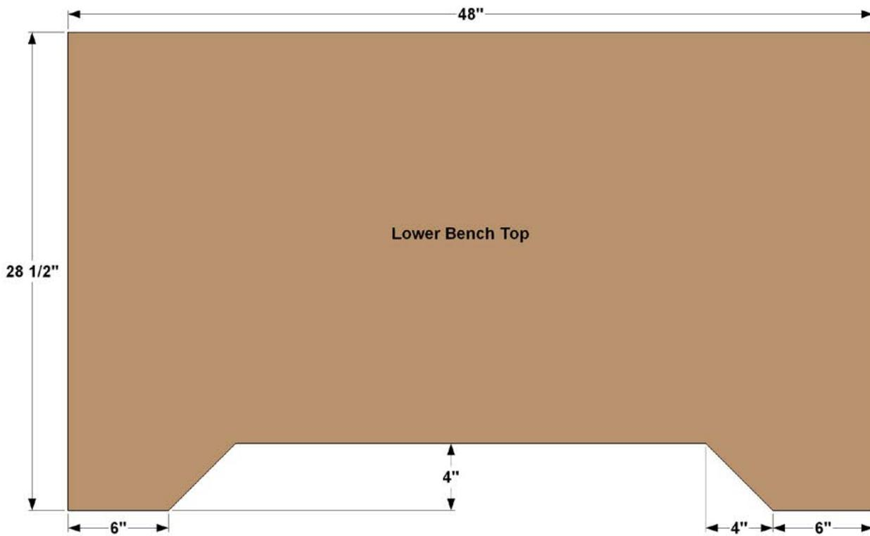
**Step 5:** Now you can create the bench top. It's made of two layers of MDF (Medium Density Fiberboard). First, cut one Lower Bench Top to size from 3/4" MDF, as shown in the cutting diagram. Then lay out and cut the recess along the front edge using a jigsaw.
